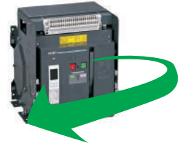
Figure 43. Remove foreign objects and dust
