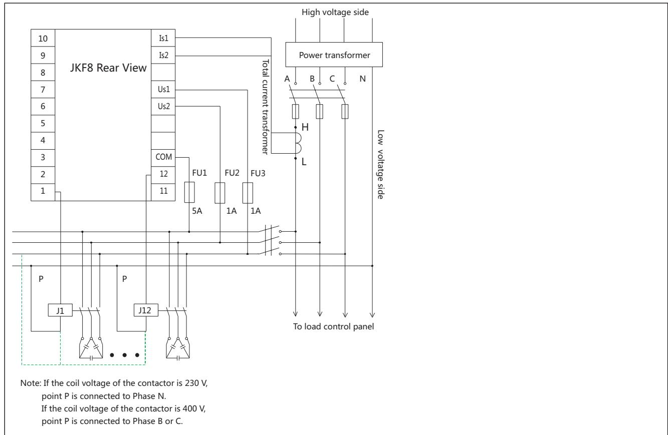
6.1 Connection terminal US1 and US2 are to be connected to the sampling voltage. AC 400 V or AC 220V shall be connected.
