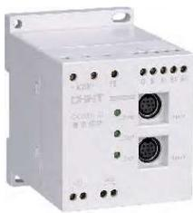
COMA-2 communication module is the interface module for our intelligent MCCB and bus communication system, suitable for NM8S series of intelligent MCCB, operating communication level conversion and relay control output. Combined with the Modbus-RTU communication protocol, the communication module can easily connect with Fieldbus master device to realize telemeter, and the remote control function.
