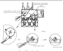
Figure 7 Operation diagram
