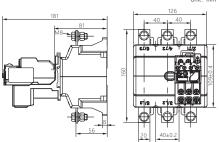
Figure 4 Overall dimensions of NR2-200
