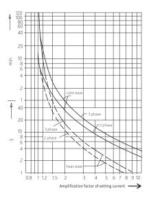
Figure 1 Thermal relay operation time - current characteristic curve
