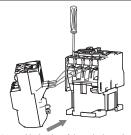
Figure 6 Assembly drawing of thermal relay and contactor
