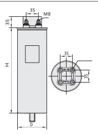
Note: The capacity of three-phase capacitor (1~8)kvar is seen in Fig.1; (10~25)kvar in Fig.2; (30~40)kvar in Fig.3;The split phase compensation capacitor has 4 connecting terminals with star connection and neutral line N lead-out, as shown in Fig.4.
