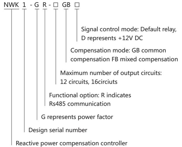
Note: When the control signal outputs +12V DC, the control object is ZCK smart combination switch or TSC thyristor switch.
