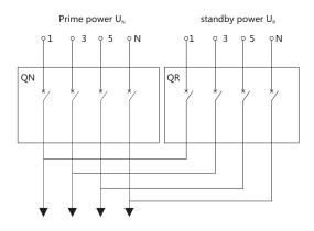
Note: QN actuator circuit breaker on the prime (normal) side QR actuator circuit breaker on the standby (reserve) side
